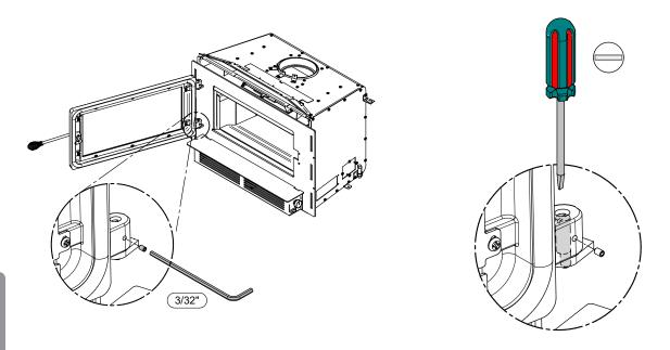
Using a flat screwdriver, turn the adjustable hinge rods in the direction shown to adjust the doors. Tighten all door hinge pressure screws when they are at the desired positions. Configurations 1-2-3-4-5-6, show in which direction these act on the adjustment of the door.
