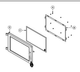
Figure 5: Replacing the glass
