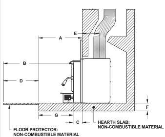
Figure 4: Additional Floor Protection - Not Raised Installation
