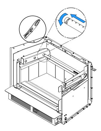
Note that secondary air tubes (A) can be replaced without removing the baffle board (B) and that all tubes are identical.
