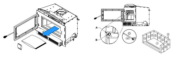
Figure 6: Empty the combustion chamber
