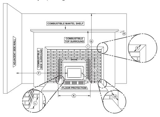
Figure 1: Hearth opening and clearances to combustibles
