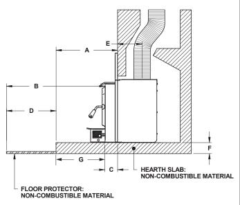
Figure 3: Additional Floor Protection - Raised Installation
