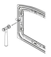
Figure 28: Installing the split pin
