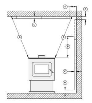
Figure 24: Heat shield clearances
