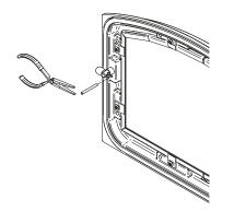
Figure 27: Removing the split pin
