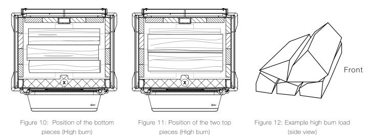
For optimal loading of a high fire, take small to medium size fuel pieces (between 2- and 3-inches cross section dimensions approximately) on the bottom and use medium to large size fuel pieces (3.5 to 4.5 inches of cross section dimensions approximately) on top. To make sure combustion is equal, put the biggest piece on top of the first three, at the front of the firebox. See an example of high burn load in the Figure 12 above.
