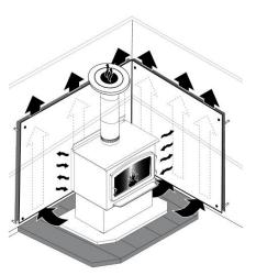
Warning: To reduce the clearances of an appliance using a single wall pipe connector, the use of a heat shield certified with the single wall pipe connector to be used as close as 6" from combustible materials must be used. Only in this case, the same clearances as a certified double wall pipe connector can be used. Refer to the booklet in the screen options to obtain the dimensions to be respected.
