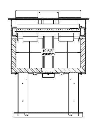
Figure 5: Front View - Combustion Chamber
