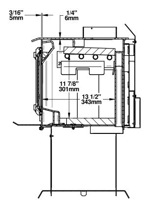
Figure 6: Side View - Combustion Chamber
