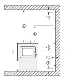
Figure 23: Heat shield clearances
