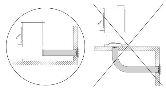
This mobile home approved stove requires the installation of a fresh air intake kit **(A)** and an insulated fresh air intake pipe (HVAC type, must meet ULC S110 or UL 181 class 0 or class 1) **(B)**, sold separately. Refer to air intake kit installation instructions for more details.
