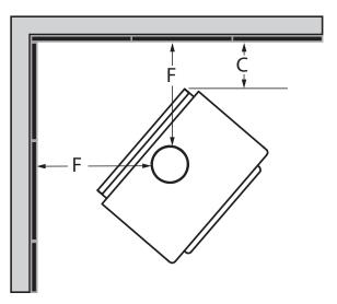
If the clearance reduction is on the same side as the door handle, position the stove at a minimum of 6 inches from the side wall (clearance B), otherwise it may be located at the clearance shown in the table above.
