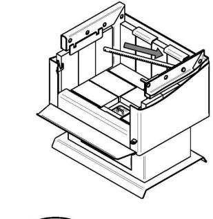
1- Starting with the rear tube, lean and insert the right end of the secondary air tube into the rear right channel hole. Then lift and insert the left end of the tube into the rear left channel.
