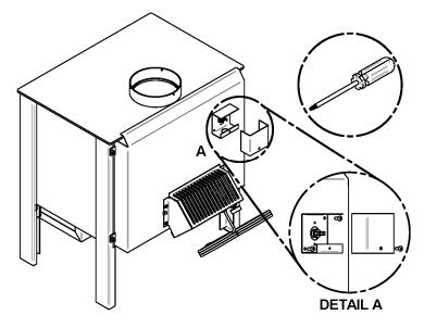
When using the optional blower, allow the stove to reach operating temperature (approximately one hour), before turning it on. The increased airflow from the blower cools the firebox and could affect the start-up combustion efficiency if the blower is turned on too early. You can also install a thermodisc to enable the blower to start or stop automatically when the stove is hot or too cold. The thermodisc part number is AC05530 for a basic model and ACO2055 for a quick connect model.
