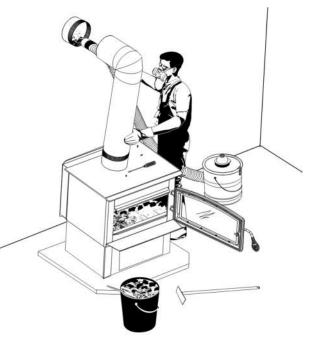
**CAUTION:** Operation of your stove without the baffle may cause unsafe and hazardous temperature conditions and will void the warranty. **NOTE:** Before installing the firebrick, check to ensure that none are broken or damaged in any way. If so, have the damaged ones replaced. Check the firebrick for damage at least annually and replace any broken or damaged ones with new ones. Inspection and cleaning of the chimney is facilitated by the removable baffle.
