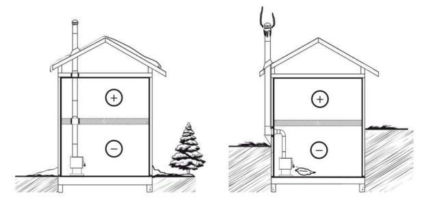
Good System Design Inside chimneys are preferred because even when no fire is burning, there is normally upward flow in the system.
