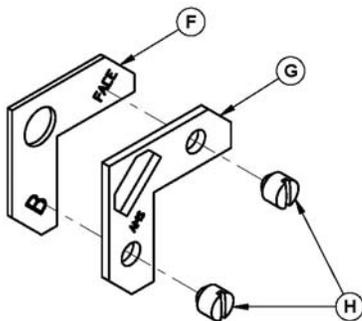
Partially thread the screws (H) on the trim's corner bracket (G) then superimpose the corner brackets (F) and (G) as shown in the image on the left.
