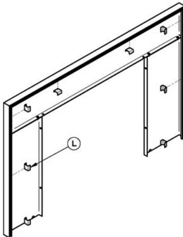
Secure the trim to the faceplate by squeezing the eight trim retainers (L) between the inner edge of the trim and the front of the faceplate. As in the image on the left.
