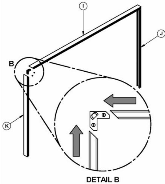
Insert the superimposed brackets (F) and (G) with the screws (H) in the groove of each decorative trim (I), (J) and (K) (see **DETAIL B**). Align the corners of the angled side of each trim, and then tighten the screws (H) to secure the trims.
