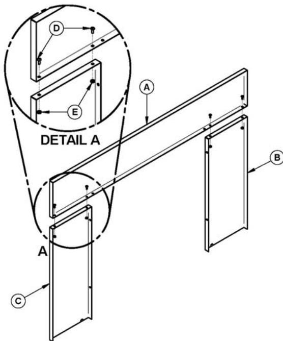
Line up the holes of the upper faceplate panel (A) with the holes of the side panels (B) and (C). Secure those together using four (4) bolts (D) and nuts (E) provided (see **DETAIL A**).
