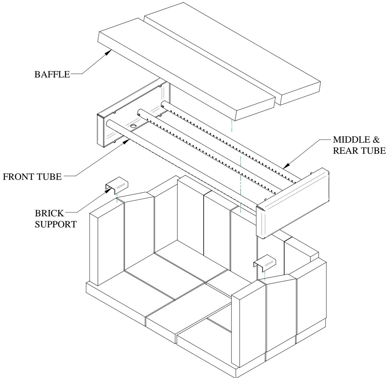
**Figure 4.4a – Baffle installation & removal for CW2500**
