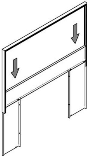
Align the trim assembly with the left and right edge of the faceplate and slowly slide it down over the faceplate.
